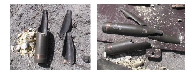
Soon thereafter both of these IM fills were then subjected to the 81mm SCJI test (RPG7 threat), the pinnacle of threat hazards that is encountered more frequently by our Soldiers fighting in support of the GWOT. Contrary to the presumption that bulk HE-filled munitions would fail such an extreme threat, one of these two candidates actually passed the 81mm SCJI with an Explosion (type-III) response -- THE ROUND DID NOT DETONATE -- a true breakthrough for insensitivity!!
